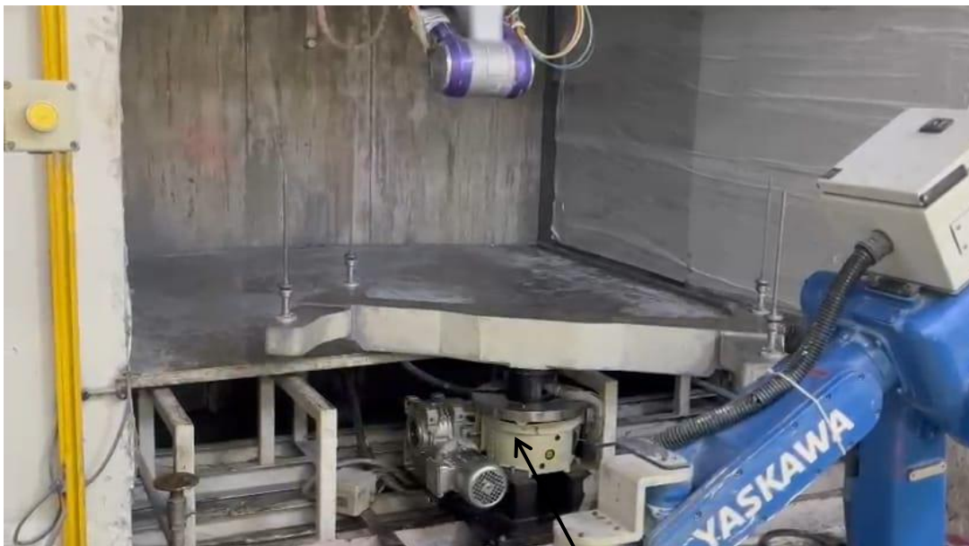
SANKYO 15AD Series Cam Indexer with ATEX Gearmotor, Base Plate, and Supporting Accessories
